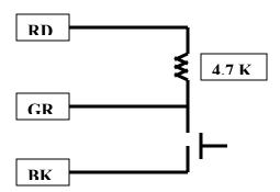
The Green lead is connected to the input bit on the I/O Card. Red is connected to +5V and Black to GND.
