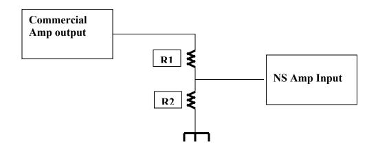
The ratio of R2 to R1 + R2 will determine the fraction of the total V sent to the NS amps. Also, the total R1 + R2 may be important because too low or high may cause problems based on input impedance of the NS amps and current that can be driven from the commercial amp (not completely clear on this but R1 + R2 on the order of 20K has been used successfully in a few different instances)
