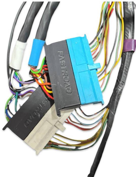
Figure 5 – FASTROAD plugs connected to the car's harness
