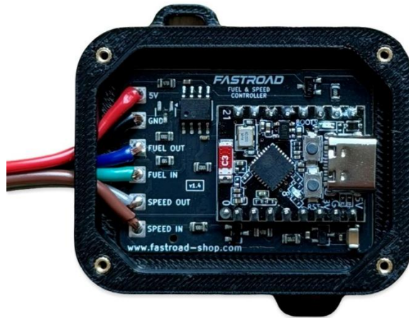
Figure 1 – Fastroad Controller board with wire labels
