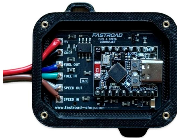
Figure 4 – Fastroad Controller board with wire labels
