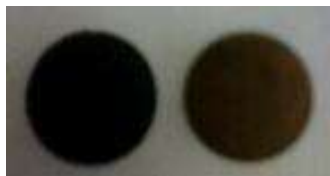
Figure 2.1.1. A picture of two pellets formed using hydraulic press.
