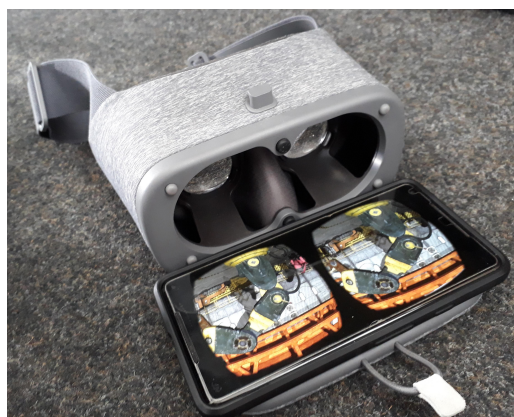
Fig. 1. Our prototype running on smartphone with Google Daydream headset showing Robot Lab scene. The smartphone renders at 2880 x 1440 resolution.
