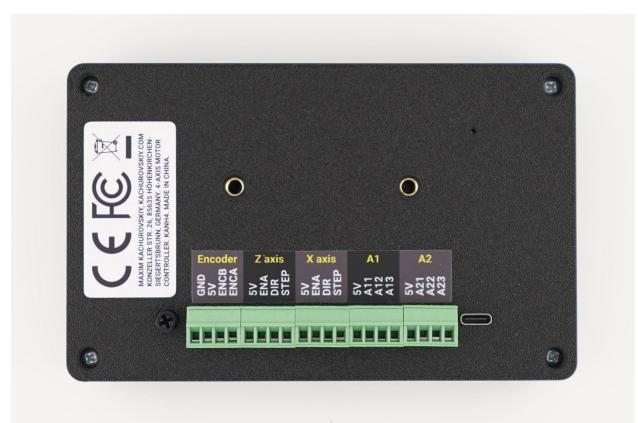
Pluggable screw terminals with 3.5mm pitch are located on the back side of the device. All terminals have ESD and short-circuit protection.
