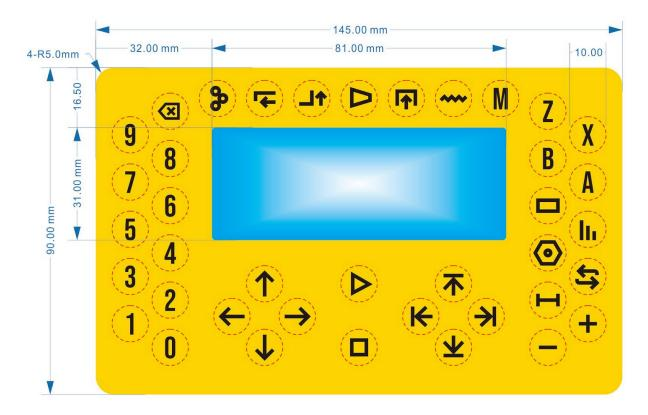
Front panel is made from 0.25mm polycarbonate with dimensions 145x90mm with 39 embossed buttons each 10mm in diameter. Attached with a double-sided adhesive tape, it can be replaced with a different one.
