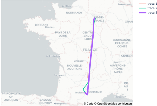
Fig. 3. Example of TS-SCAN with d = 0.05 and min_{elements} = 10 on a sample of ADS-B Trajectories.
