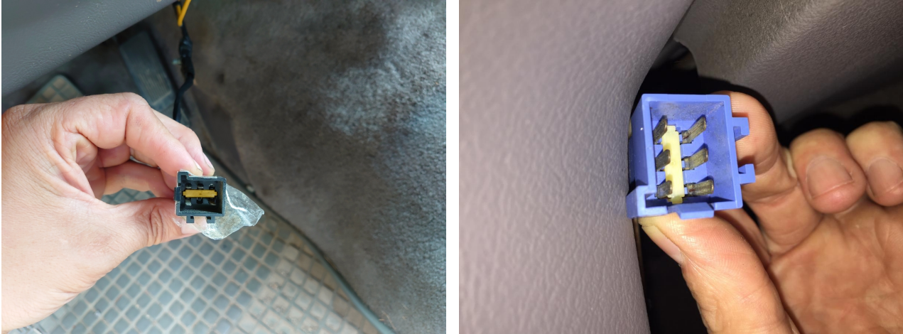
Figure 4. Two types of body connectors.
