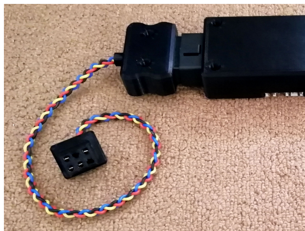
Figure 6. Body connector adapter cable connected to the scanner.
