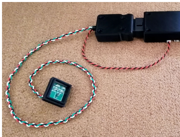
Figure 8. Engine connector adapter cable connected to the scanner.
