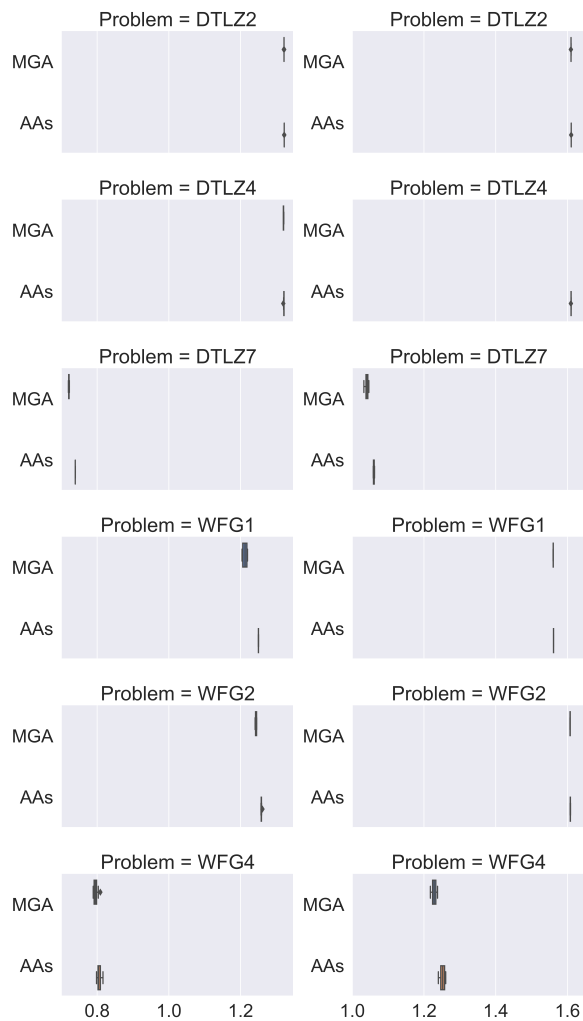
Fig. 7. Boxplots depicting hypervolume values ( x axis) achieved by truncated reference fronts using different archivers ( y axis). Left: M = 3 ; right: M = 5 .
