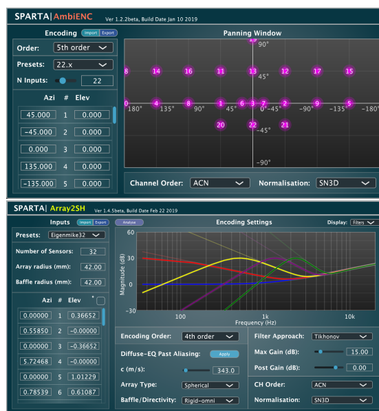
Fig. 3: Monophonic (top) and microphone array (bottom) ambisonic encoders.
