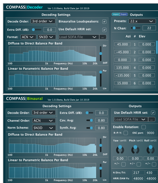
Fig. 10: Parametric Ambisonic decoder plug-ins.
