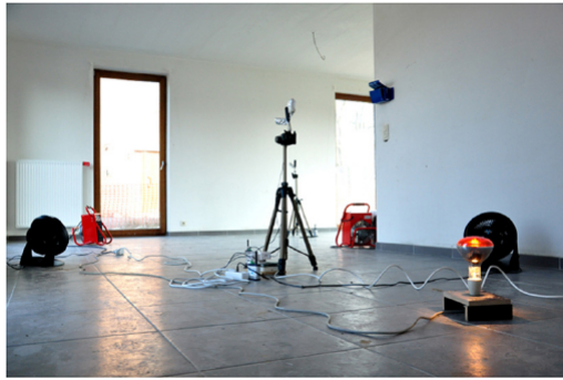
Figure 1.3: Setup of a co-heating test [BR14]
