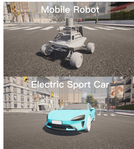
Figure 14: Custom assets imported into CARLA-Air through the extensible asset pipeline. Top: a four-wheeled mobile robot with onboard LiDAR, imported from an external FBX model. Bottom: a custom electric sport car with user-defined vehicle dynamics. Both assets operate within the shared simulation world alongside all built-in CARLA traffic and AirSim aerial agents, and are visible to all sensor modalities.
