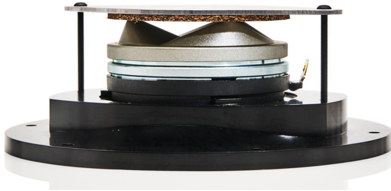
Figure 7: Photo of the R2904 tweeter mounted on the waveguide using a clamp.
