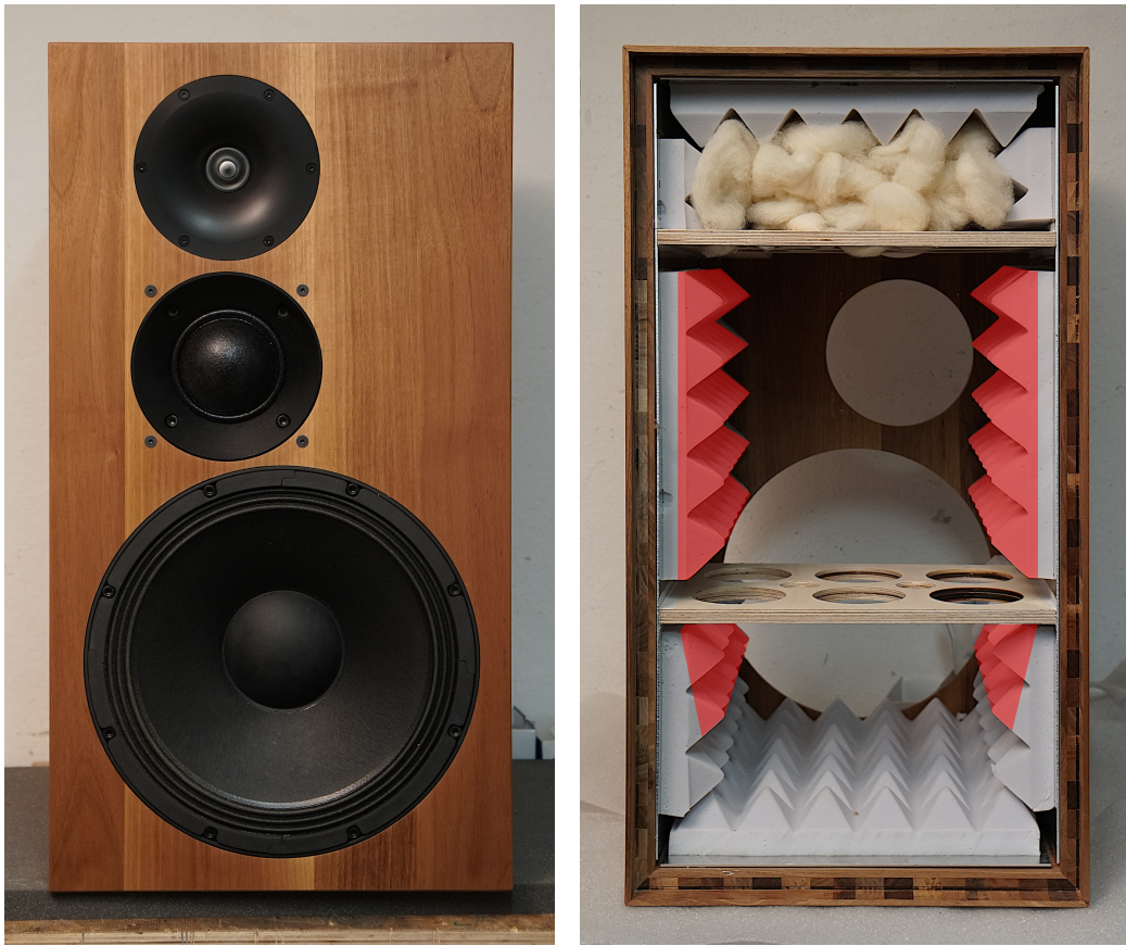
Figure 6: OSMC front and back with rear wall removed to show the bracing and damping. The red parts of the Basotect absorbers are removed using a large knife.
