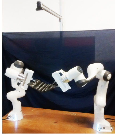
Fig. 1. View of our experimental setup during testing of bi-arm visual shape servoing of a rubber tire tread with an overhead monocular camera.
