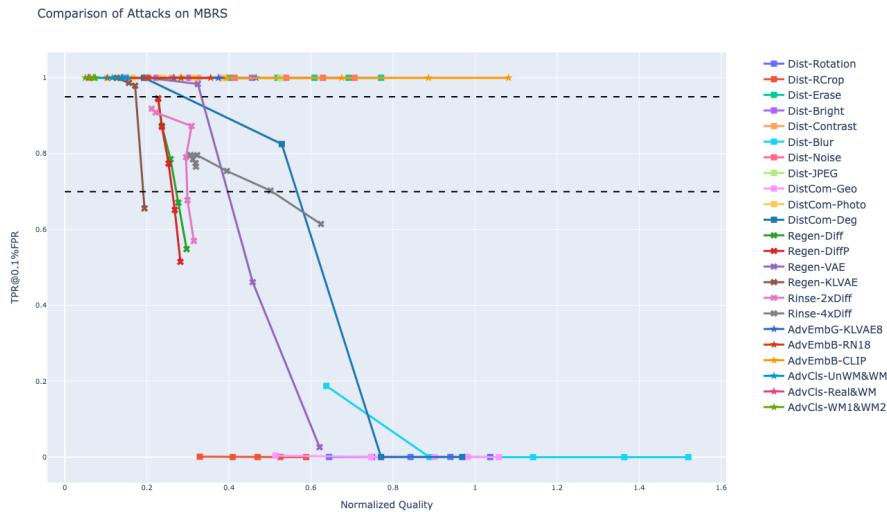
Figure 32. Stress test results for MBRS. It is vulnerable to certain distortion attacks (resized-cropping, blurring, rotation, combo distortions) and regeneration attacks, but robust against other distortions (JPEG compression, brightness/contrast, random erasing, noise) and adversarial attacks.
