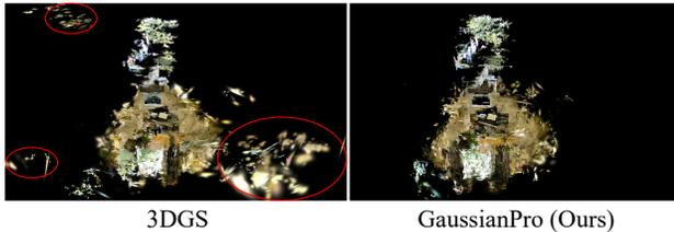
Figure 7: Visualization of Gaussians in the *Room* scene of MipNeRF360 dataset. Our method contains fewer noisy Gaussians and achieves a more compact representation.
