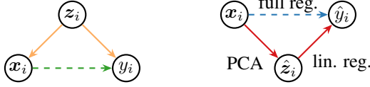
Figure 2: Model definitions. Left: Data-generating models: Latent factor model (orange) and equivalent direct model (green). Right: Estimation models: PCR (red) and full regression model (blue).
