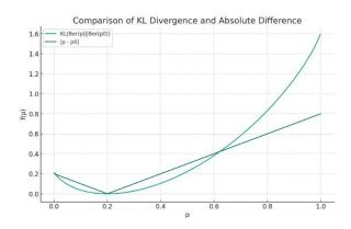
Figure 26. Comparison of KL regularization and pointwise centered  $\ell_1$  regularization for a scalar value. Around the prior value  $p_0$ , the KL is much smoother than  $\ell_1$  regularizer.  $f'(p) = \log\left(\frac{\frac{p}{1-p}}{\frac{p}{1-p_0}}\right) \text{ for KL, which is very close to 0 when } p \in [p_0-\epsilon, p_0+\epsilon]. \text{ However, for } \ell_1 \text{ regularization, } f'(p) = 1 \text{ or } -1 \text{ for all points except } p = p_0.$
