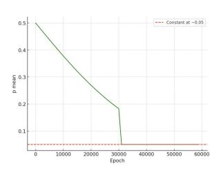
Figure 25. Mean of p across various epochs when the regularization used is  $|mean(p) - \frac{s}{d}|$ . In this particular experiment,  $\frac{s}{d} = 0.05$ .
