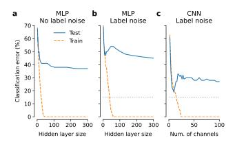
Figure 5: Deep double descent in MNIST-1D classification. Here the test set had 12 000 samples. (a) MLP classifier with one hidden layer. (b) MLP classifier; 15% label noise. (c) CNN classifier with three convolutional layers; 15% label noise. Adapted with permission from Prince (2023, Section 8.4). CPU runtime:  $\sim 60$  minutes. [CODE]
