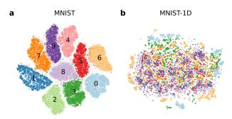
Figure 3: Visualizing the MNIST and MNIST-1D datasets with t-SNE. The well-defined clusters in the MNIST embedding indicate that the classes are separable via a simple kNN classifier in pixel space. The MNIST-1D plot reveals little structure and a lack of clusters, indicating that nearest neighbors in pixel space are not semantically meaningful, as is the case with natural image datasets. [CODE]
