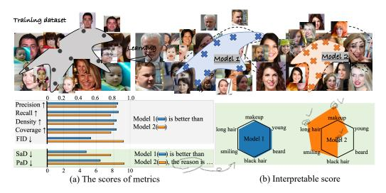
*Figure 1.* Conceptual illustration of our metric. We design the scenario, Model 2 lacks diversity. (a) Although existing metrics (gray box) capture the inferiority of Model 2, they do not provide an explanation for the judgments. (b) Our attribute-based proposed metric (green box) has an interpretation: Model 2 is biased regarding long hair, makeup, smiling, and beard.
