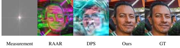
Figure 1. Illustration of the results of noiseless 4\times oversampled phase retrieval. RAAR produces restoration with misaligned channel orientation, DPS (Chung et al., 2022a) generates deviated solution, while ours produces much better solution.
