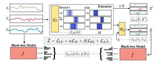
Figure 2. The overall architecture of TIMEX++, which consists of the explanation extractor and the conditioner generating new instances.
