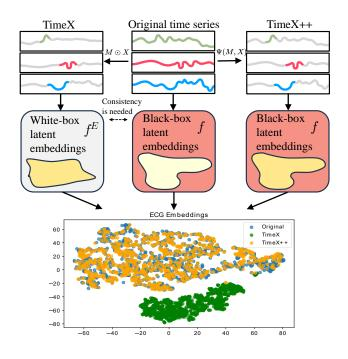
*Figure 1.* A comparison of our model and the reference model, where the latent embeddings of explanations are learned from the ECG dataset. Our explanations are within the original distribution, whereas explanations of the reference model are not.
