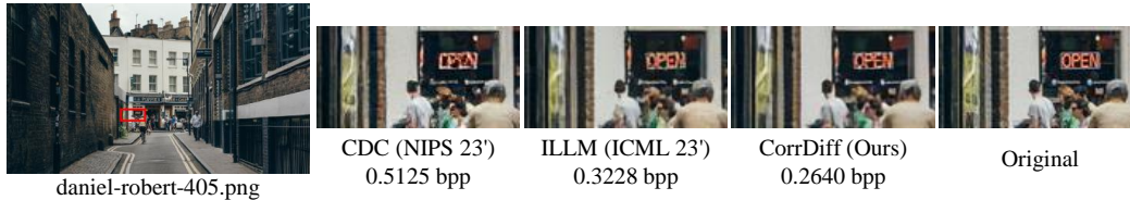
Figure 1. Visual results compared to CDC (Yang & Mandt, 2023) and ILLM (Muckley et al., 2023). The patch is cropped from daniel-robert-405.png from CLIC professional dataset (Toderici et al., 2020). [Zoom in for best view]
