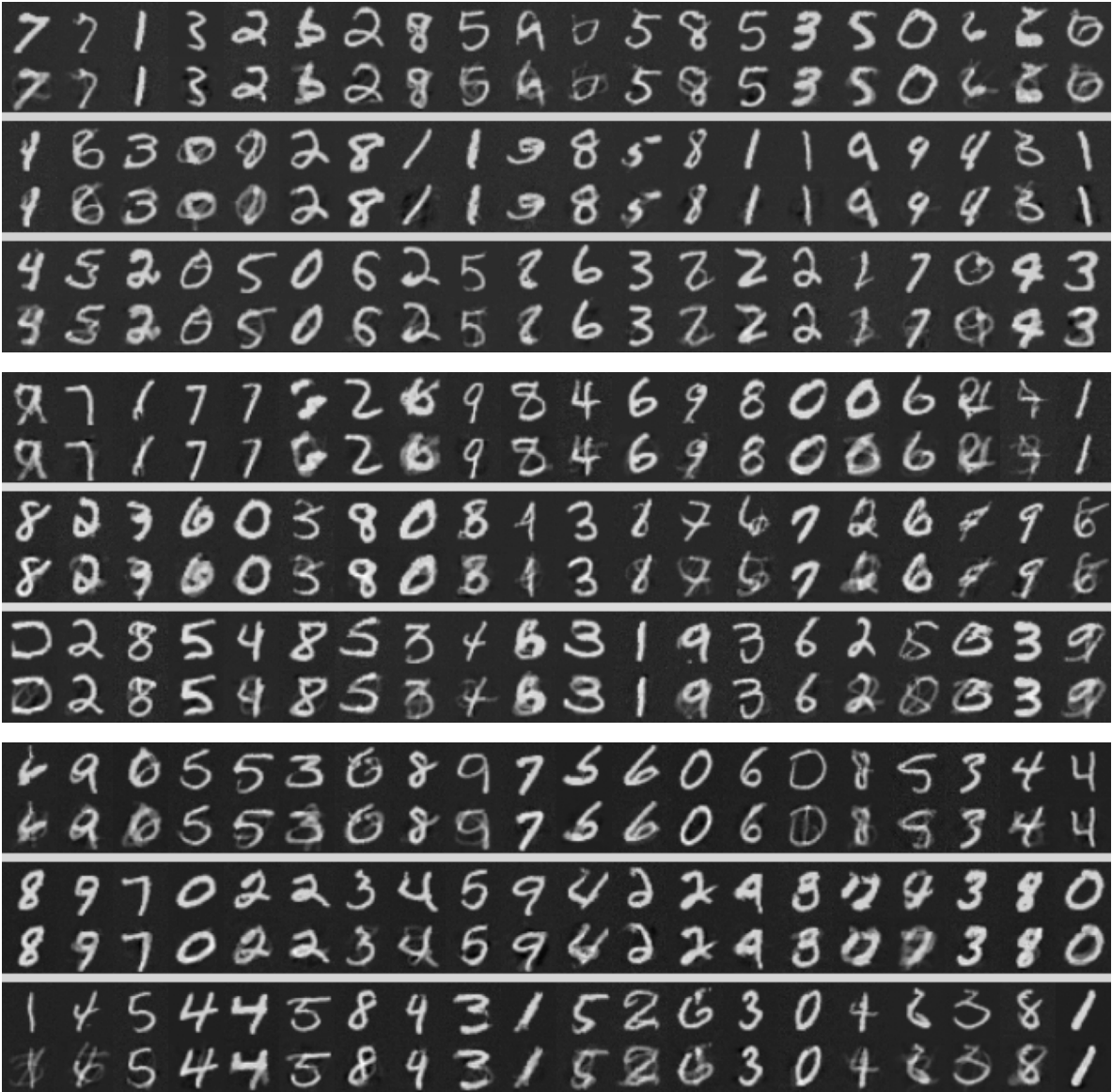
Figure 3. MNIST 32x32 image generation. Every top row is the integration of the corresponding ODE via Dormand-Prince's 5/4 method, which makes 108 function evaluations. Every bottom row corresponds to single function evaluation approximation.
