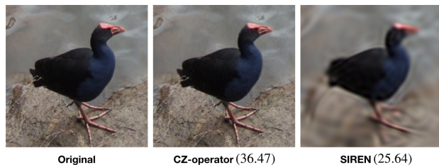
Figure 7. The CZ-Operator in O-INR can successfully represent images with high PSNR values.
