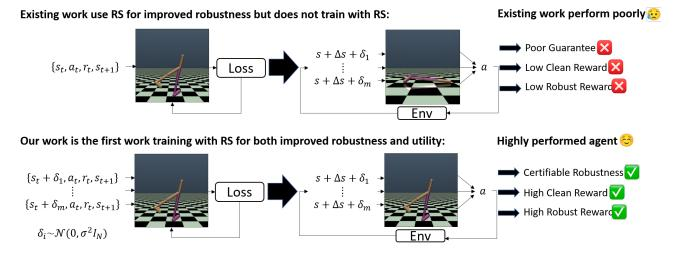
*Figure 2.* The overview of our framework. We propose new DRL training algorithms leveraging Randomized Smoothing, achieving strong certifiable robustness, high clean reward, and high robust reward simultaneously.
