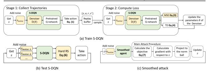
*Figure 3.* The flow chart of: (a) training process of S-DQN, (b) testing process of S-DQN, (c) our Smoothed Attack pipeline for smoothed agents, which is much more effective than non-smoothed attack.
