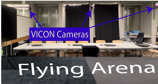
Figure 21. The D-FALL Laboratory of ETH Zürich, consisting of a dedicated Flying Arena and 5 (3 shown) mounted VICON Cameras for state estimation.
