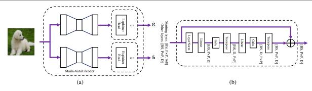
Figure 10. Transferable explainer architecture. (a) Explainer architecture. (b) FFN-layers for the explainer head.
