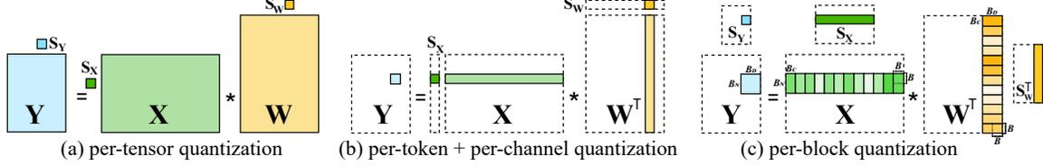
Figure 4. Different quantization methods for linear layer.
