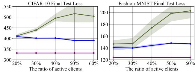
Figure 13: The mean final loss values of FedAST (blue), FedAST-NoBuffer (olive green) and centralized training (violet) with varying active client ratio, when training 3 identical models. The left figure is for CIFAR-10 dataset, while the right figure is for Fashion-MNIST dataset. With a higher number of active clients, thanks to the buffer, FedAST remains its performance while FedAST-NoBuffer gets worse.
