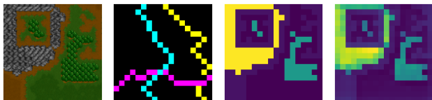
Figure 3: Algorithm 3 gets several images and paths as training data to reconstruct the grid costs with the trained Resnet18.
