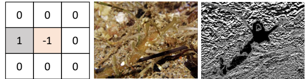
Figure 2: Examples of our BCNN layer. The left is a sample of 3 \times 3 BCNN layer, the center is the input image, and the right is the output of the BCNN layer. Our BCNN is a fixed-weight binary convolution layer that can provide the comparison information of neighboring pixel pairs. Our results show that BCNN can provide a precise boundary for a given image.
