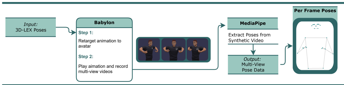
Figure 8. Pipeline for producing the synthetic animation data with Babylons.js and MediaPipe. The chart showcases the multi-view recordings captured of the Ready Player Me Avatar.
