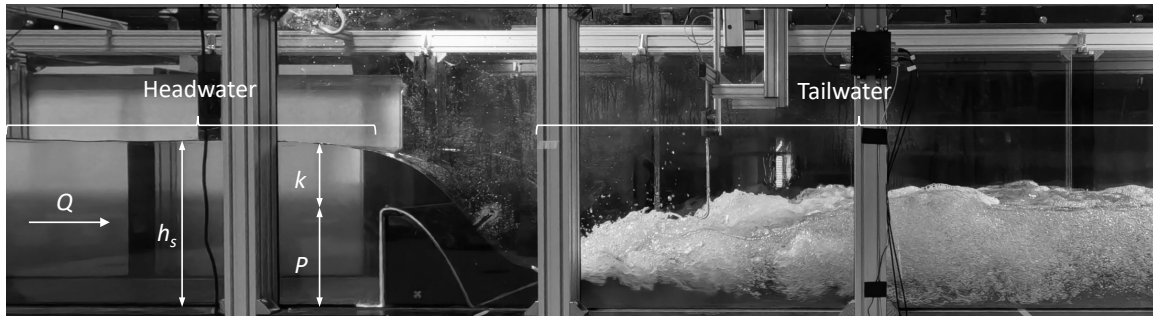
Figure 1: Example of flow behavior over an exemplary linear weir geometry with the weir height P and the overfall height k in a scaled physical model test with flow direction from left to right.
