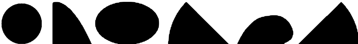
Figure 10: Six additional weirs of the dataset FlowProp-Diverse. From left to right: Circle, Ogee, Ellipsoid, Tilting Left, Hose and Tilting Right.
