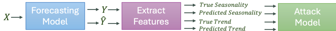
Figure 1: Flowchart illustrating the process from the initial forecasting model to the final attack model, highlighting how extracted features are used for MIAs.
