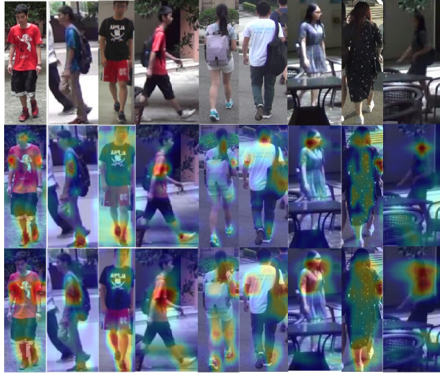
Figure 5: Example of the attentive feature maps. The first row is the original image, the second and third rows are the outputs of the global and fusion branches.
