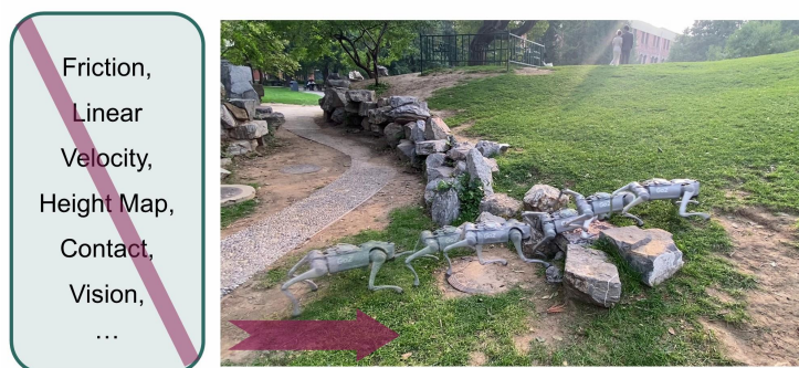
Figure 1: We propose a framework for training a robust quadruped locomotion policy without relying on privileged information. The robot effectively navigates challenging terrains, showcasing adaptive locomotion skills acquired through self-learning.
