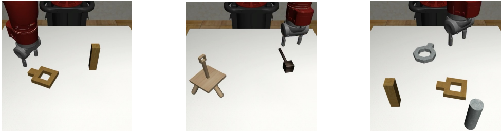
Figure N.1: Data Generation for Sawyer Robot Arm. Example configurations for task variants where SkillGen generated data for the Sawyer robot arm, using source human data collected on the Panda robot arm.
