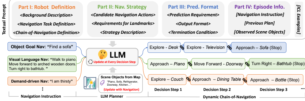
Figure 2: The workflow of Dynamic Chain-of-Navigation (DCoN). Different types of navigation instructions can be unified into DCoN by LLM. The next action and landmarks will be updated based on observed scene objects at every decision step. Beyond extracting actions and landmarks, DCoN achieves semantic label alignment, common-sense reasoning, and environmental exploration for navigation planning. Complete prompt and output examples are shown in Supplementary Materials .
