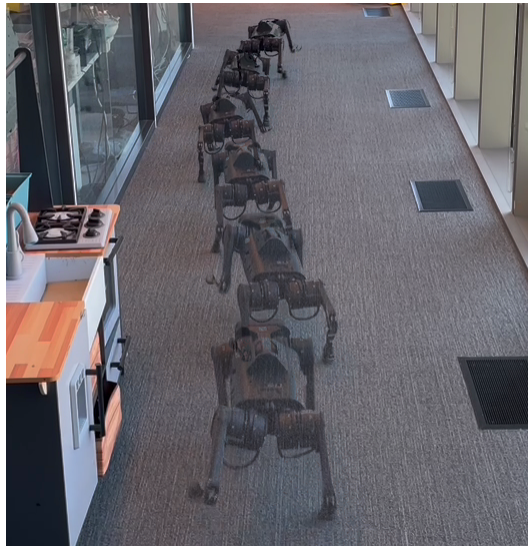
Figure 7: Real-World Deployment. Frame overlay demonstrating the deployment of the BoT walking policy to a Unitree A1 quadruped robot.
