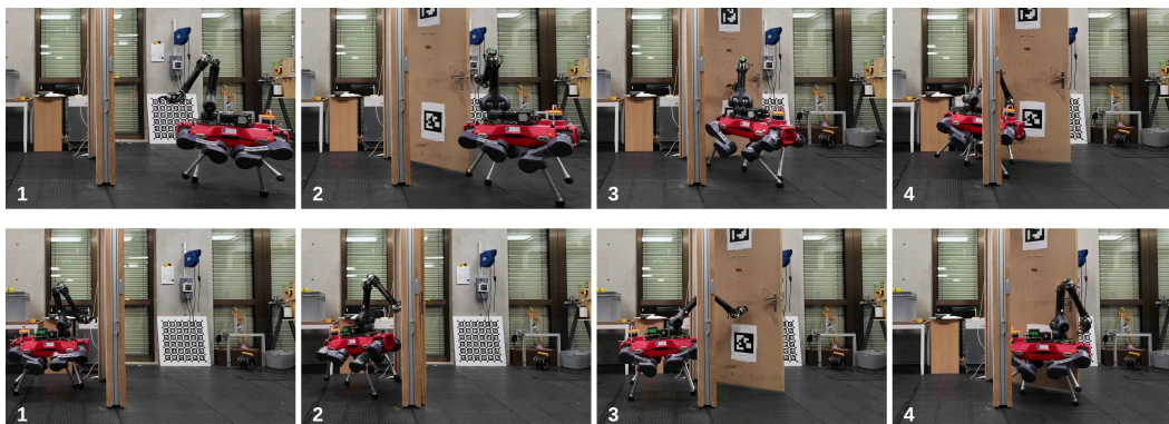
Figure 1: We present a control policy that can open and pass through both pull (top) and push (bottom) doors by estimating the door properties during deployment.
