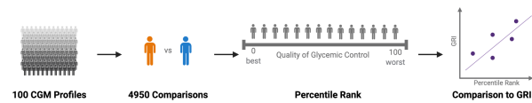
Figure 1: Assessing LLM alignment to the GRI. Each dataset had 4950 pairwise comparisons of every profile. Each of the 100 profiles was given a rank based on the number of other profiles the LLM decided that it was better than. This percentile rank was then compared to the GRI.
