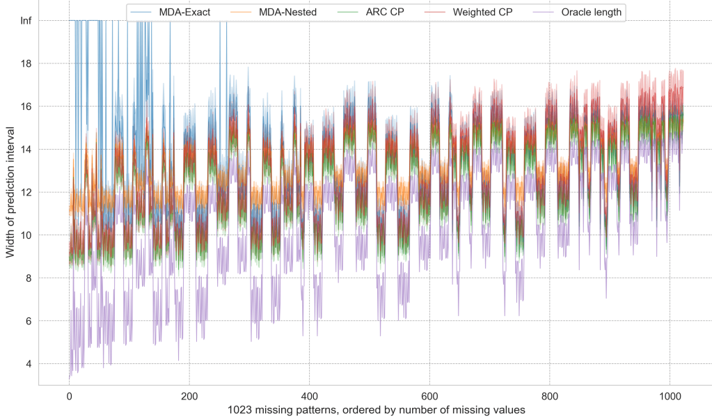
Figure 13: Synthetic dataset with 20% missing values and independent features: mean and 99% confidence interval of prediction interval width with respect to 1023 missingness patterns, comparison for whether using correction method.
