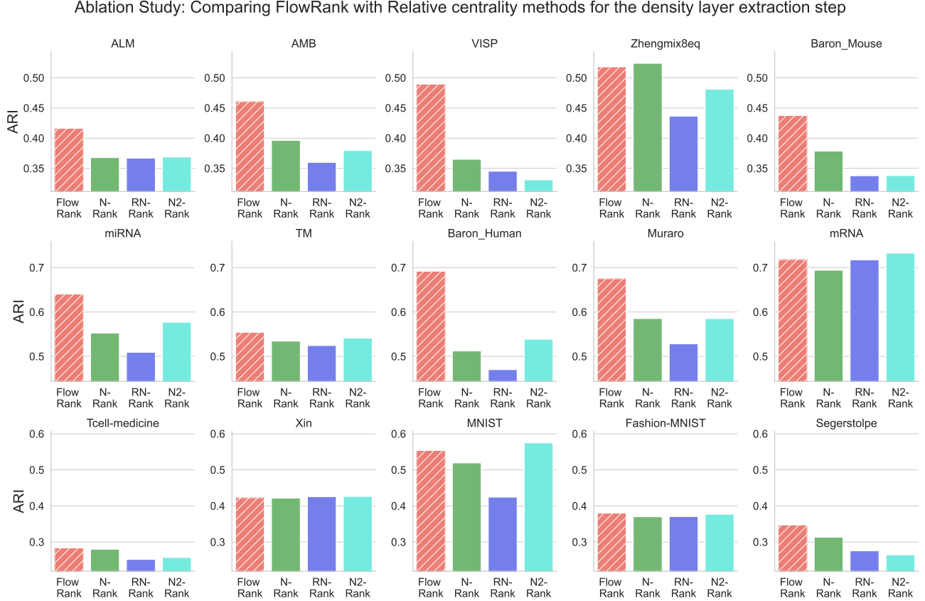
Figure 10: Contrasting the performance (ARI) of FlowRank with that of Relative centrality methods in the density-layer-extraction step of CoreSPECT. In 11 out of 15 datasets, FlowRank produces the best result, and is within 2% of the best in the other four datasets.
