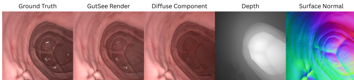
Figure 4: An example of light-geometry decoupling. Our physically based scene representation and explicit coaxial light model separates lighting effects from the underlying scene geometry.
