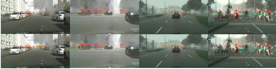
Figure 4. Detection results before (top) and after (bottom) adaptation. Green circles show new correct detections, while yellow circles show false positives removed by FogTTA.
