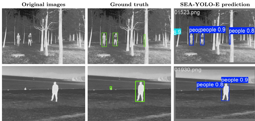
Figure 4. Object detection success scenario from M3FD dataset (2nd row: Occluded object detection success scenario - the SEA-YOLO-E with self-supervision pretraining succeeds to detect people instances in a highly occluded case. 3rd row: Distant object detection success scenario - the SEA-YOLO-E with self-supervision pretraining succeeds to detect very small people instances in a distant case.
