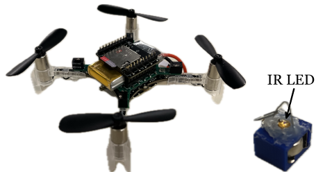
Figure 2: Hardware used for experiments. We rely on a Bitcraze Crazyflie 2.1 with standard motors, Micro-SD-card extension, and custom RPM measurement board that uses IR-LEDs. These LEDs can also be tracked by a motion capture system. The payload is equipped with another active IR LED for tracking.
