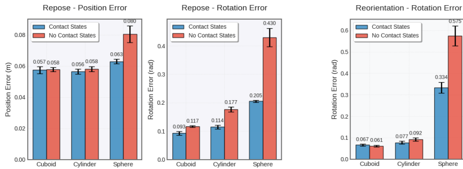
Figure 7: Tracking error comparison on unseen object shapes across various tasks. We compare our contact-explicit policy (uses contact states) with a baseline policy that uses one-hot task encoding (no contact states) to represent the task. Results are averaged over 1000 episodes, each lasting 20 seconds of simulated time.
